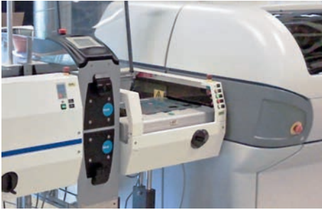
SMT contact clean machine installed prior to DEK screen-printer
