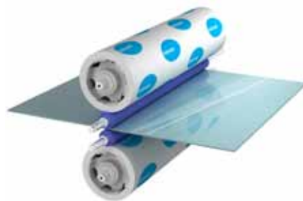
With contact cleaning, two tacky rubber rollers lift contaminants off both sides of the PCB at once. The rubber rolls then pass off the contaminants to the adhesive rolls.
