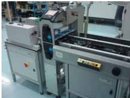
A bare board is fed into a contact cleaning system at the start of an automated production line to remove surface contamination prior to the stencil printing process.
