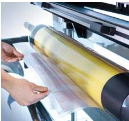
Bobst Expertcut 106 PER Demounting the plate after the print job
