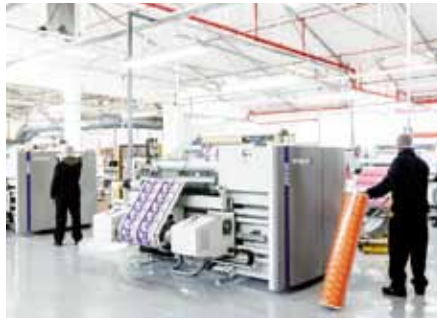
Redevelopment of the CTP flexibles Cape Town site has resulted in a 5000m² slitting hall where seven of the ten slitter rewinders are Titan machines
